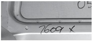
On a pre-4200 VIN car, locating the key code for the ignition is very hit or miss. It is very unlikely to be found on the stainless under the headliners, but it is possible that DMC (Texas) might have it on file. If not, the key codes for the ignition were also written on a small label that was affixed to the bottom of the steering column canopy as shown in the photo. Many of these have faded, fallen off or been removed over the years, so you may find nothing there.
